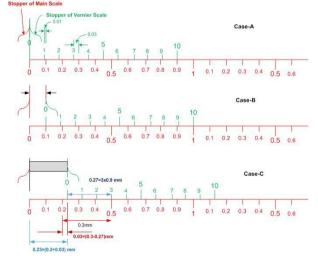
There could be situation where none of the divisions of VS match with any mark on MS and this involves application of Rounding of numbers discussed at para 1.2.4 Significant Digits.
