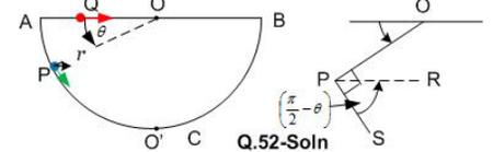
below center of the bowl O, and then while traversing upward its velocity decreases. The increase in velocity of P, while sliding down increases its horizontal velocity  $v$  and on reaching back to B at height of A, it comes back to  $v$ . Thus all along traversing semicircular arc ACB its horizontal velocity  $v_h > v$  and hence time taken by P to reach B would be  $t_p < t_q$ . **Answer is Option (a)**
