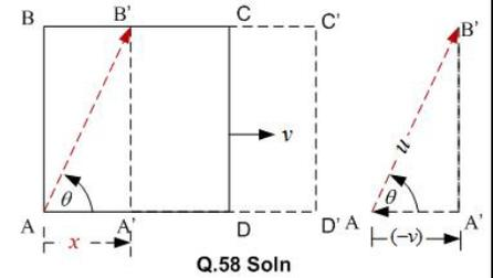
after projected from point A with a speed  $u$  at an angle  $\alpha$  so as to hit the vertex B. Relative velocity of particle w.r.t. frame should be such that its horizontal component should lead to cancellation of relative velocity of frame, i.e.  $u \cos \theta - v = 0 \rightarrow \cos \theta = \frac{v}{u} \rightarrow \theta = \cos^{-1} \left( \frac{v}{u} \right)$ . **Answer is Option (b).**
