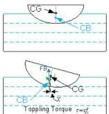
**Situation b)** In this CG of Object is above CB. When the object is tilted in any direction, say clockwise, the CB would also shift clockwise and  $F_b$  would compound turning torque, on the object about CG, and this is called **Toppling Torque**. This is a cascading effect in same direction until the object topples and sinks. Such a situation is called **dynamic inequilibrium**.
