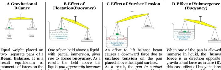
moments of forces on the beam to keep it horizontal. Thus equal weights are measured equal.
