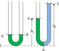
$\rho_2$  is such that  $\frac{\rho_1}{\rho_2} = \frac{h_2}{h_1}$ . This observation lays foundation in understanding of fluid mechanics in general and fluid statistics in particular.
