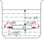
direction. Since,  $\vec{F}_g$  is vertical downward and passes through its COM, therefore,  $\vec{F}_b$  must also pass through COM and in vertically upward direction.
