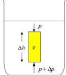
$\rho g \Delta h = \Delta p$ , or  $\frac{dp}{dh} = \rho g$ . Therefore, net vertical pressure at a depth is  $p = \int (\rho g) dh + C =$  $\rho gh + C$ . Here, C is integration constant such that at h = 0, i.e. on the surface of the liquid pressure is  $p_0$ , and, thus using these values in the instant integration we arrive at  $C = p_0$ . It implies that at any depth h
