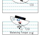
Shift in CB depends more upon shape of the floating objects, which are generally symmetrical about vertical axis in its static equilibrium. But, shift in CB requires to be observed closely, which generally conforms to the above analysis.
