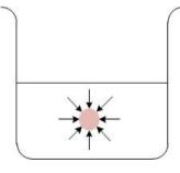
immersed in liquid below the surface of liquid in the vessel. It will be observed that the ball remains in place. It implies that the fall is in equilibrium which is possible only if resultant force acting on the ball along any line drawn through it the ball is Zero. Now, let a thin
