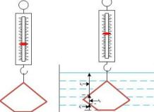
**Stability During Float:** Extending the Archimedes principle, together with principle of *Centre of Gravity (CG)* and moments. Mass distribution of floating object is different and may be non-homogenous, while mass distribution of homogenous displaced liquid is based on volume immersed. This could lead to three situations.
