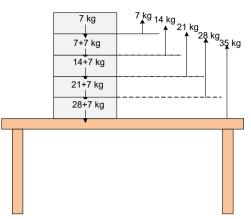
weighing 7 kg kept on the table, as shown in the figure, is  $F = 7 \times 5 = 35$  kg. The stack remains in place unless it is displaced. Force exerted by each box, progressively, on the lower box and reaction offered by the lower surface is shown in the figure.
