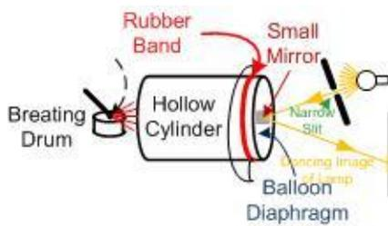
tightened with a rubber band. A small piece of mirror is pasted on balloon such that a light ray through a slit creates a image on a wall. As the beating of drum starts at open end of hollow cylinder, the image starts dancing. The simple reason is the pressure waves create a vibration in diaphragm. This vibration changes position of image as per laws of reflection, to be elaborated in light waves. Beating drum sets in
