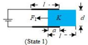
**State 2:** The slab remains accelerated until it fill gap completely as shown if figure (ii), and by then acquires velocity as per Third Equation of Motion  $v^2 = 2ks \Rightarrow v = \sqrt{2ks} \Rightarrow v_{max} = \sqrt{2 \left( \frac{\epsilon_0 bV^2(K-1)}{2dm} \right) (l-a)} = \sqrt{\left( \frac{\epsilon_0 bV^2(K-1)}{dm} \right) (l-a)}$ . At this state when gap is completely filled force on the dielectric becomes zero.
