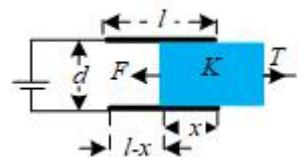
This system is equivalent to a parallel combination of capacitors  $C_1$  and  $C_2$  having an equivalent capacitance  $C = C_1 + C_2 \Rightarrow C = \frac{\epsilon_0 KAx}{ld} + \frac{\epsilon_0 A(l-x)}{ld} \Rightarrow C = \frac{\epsilon_0 A}{ld} (Kx + l - x) \Rightarrow C = \frac{\epsilon_0 A}{ld} (l + (K - 1)x)$ . Accordingly,
