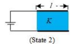
**State 3:** In state 2, under inertia as per Newton's First Law of Motion would continue with the instantaneous velocity to create gap on right side and experience electrostatic force  $F_3 = F_1$  i.e. of same magnitude but in opposite direction which would retard the slab until it reaches state 3.
