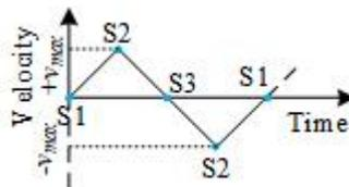
Considering the three states the slab would continue perform a periodic motion in the system where effect of friction and gravity is ignored. Thus, transition of slab from one state to the other is shown in the figure where at  $t = 0$  the slab is in state 1 (S1), at  $t = \frac{T}{4}$  the slab is in state 2 (S2). at  $t = \frac{T}{2}$  the slab is in state 3 (S3). at  $t = \frac{3T}{4}$  the slab is in state 2 (S2) and at  $t = T$  the slab is back in state 1 (S1).
