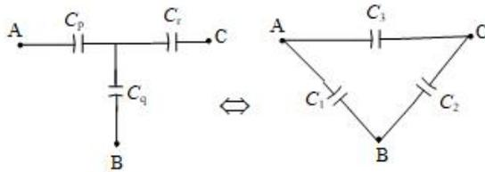
This star connection is shown in the figure and is required to be converted into an equivalent delta connection of capacitors  $C_1$ ,  $C_2$ , and  $C_3$ . As
