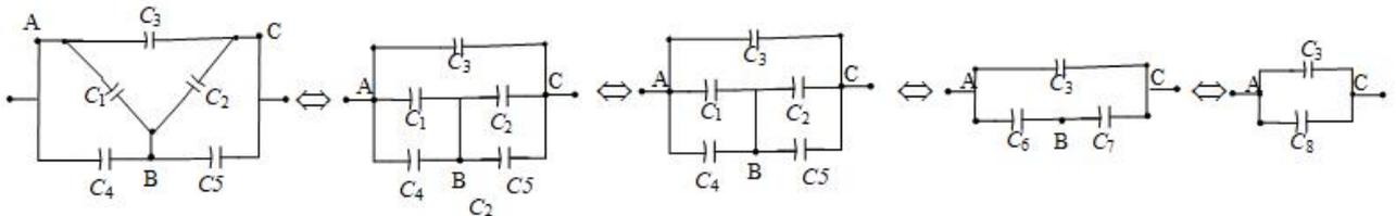
Accordingly,  $C_6 = C_1 || C_4 \Rightarrow C_6 = 0.5 \times 10^{-6} + 3 \times 10^{-6} \Rightarrow C_6 = 3.5 \times 10^{-6} F$ .
