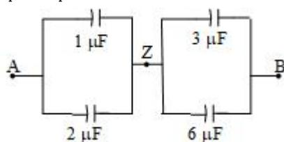
This is a pair of parallel combination between A-Z such that  $C_1 = 1 \times 10^{-6} + 3 \times 10^{-6} \Rightarrow C_1 = 4 \times 10^{-6}$  and between Z and B such that  $C_2 = 2 \times 10^{-6} + 6 \times 10^{-6} \Rightarrow C_2 = 8 \times 10^{-6}$ .
