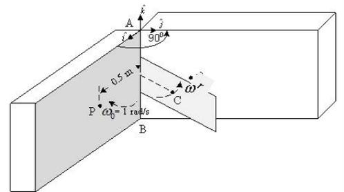
Likewise, angular impulse, about line AB, caused by impact of the laminar on rubber stopper P would be  $\Delta L = \Delta P(0.5) = I\Delta\omega \rightarrow 6(0.5) = (I_C + Mr^2)(1 + \omega) \rightarrow 3 = (1.2 + 30r^2)(1 + \omega)$ . This with the vale of  $\Delta P$  calculated above transforms into  $3 = (1.2 + 30r^2) \left( \frac{1}{5r} \right) \rightarrow 30r^2 - 15r + 1.2 = 0$  is a quadratic equation with
