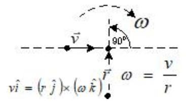
$$\omega = \frac{v_{2,1}}{r} = \frac{\pi \times 10^4}{3 \times 10^4} = \frac{\pi}{3} \text{ rad/hour which translates into standard unit } \frac{\pi}{3 \times 60 \times 60} = 3.0 \times 10^{-4} \text{ rad/s. This is part (b) of the answer.}$$
