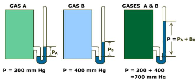
**Partial pressure in terms of mole fraction:-** Mole fraction is a method of expressing concentration of a substance in a mixture as a fraction of total moles of all substances. If  $n_1$  moles of any substance are present in  $n$  moles of the mixture, then mole fraction  $x_1$  of the substance,  $x_1 = \frac{n_1}{n}$ , for example, for a mixture of two substances A + B having moles  $n_A$  and  $n_B$  respectively, then their mole fractions are:
