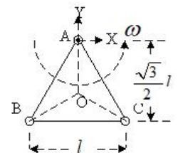
the centripetal force exerted by the hinge shall be  $F_c = (3m)r\omega^2$ . Accordingly,  $F_c = 3m \frac{l}{\sqrt{3}} \omega^2 = \sqrt{3}ml\omega^2$ ,
