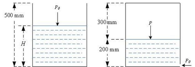
This is the instance when pressure at the orifice is in equilibrium such that  $p + \rho g (0.2) = p_0 \rightarrow p = p_0 - 0.2 \rho g = 10 \times 10^5 - 0.2 \times 10^3 \times 10 = 998 \times 10^3$ . Moreover, the drain being
