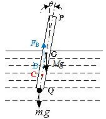
I-24 Let A is the area of cross-section of the cylinder, and h is its height. Therefore, mass of the cylinder is  $M = AH\rho = 0.8Hh$ . Mass of the liquids displaced  $M = A(h_A\rho_A + h_B\rho_B) = A(0.7 \times 1.2 + 1.2 \times 0.8) = 1.8A$ . Equating the two  $M = 0.8AH = 1.8A \rightarrow H = \frac{1.8}{0.8} = 2.25$  cm. Therefore length of the cylinder in the air is  $h = H - (h_A + h_B) = 2.25 - (1.2 + 0.8) = 0.25$  cm. This is answer of part (b).
