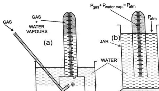
When the water level inside the container becomes equal to outside level then,  $P_{\text{atm}} = P_{\text{total}}$  (equal to pressure of gas + water vapours) =  $P_{\text{Oxygen gas}} + P_{\text{H}_2\text{O}}$ ,  $\therefore P_{\text{O}_2} = P_{\text{atm}} - P_{\text{H}_2\text{O}}$  ( $P_{\text{Water}}$  = pressure due to water vapours is called aqueous tension),  $P_{\text{Dry gas}} = P_{\text{Moist gas}} - \text{aqueous tension } (t^\circ\text{C})$ .
