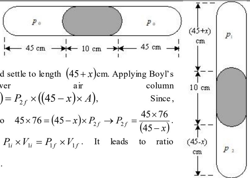
expansion in upper air column and it would settle to length  $(45 + x)$  cm. Applying Boyle's law to lower air column
